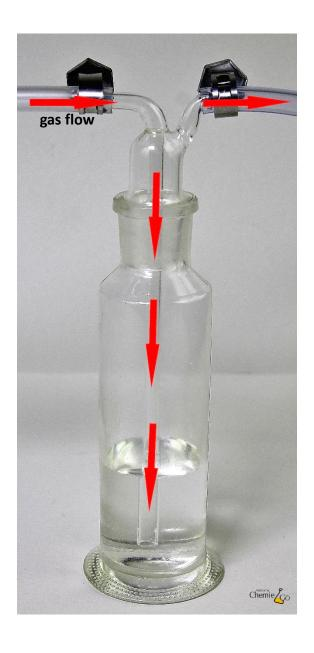
When using an absorbent (chemical purification) the correct flow direction of the gas is important.
